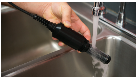
Rinsing membrane cartridge (still connected to probe) under running water.
