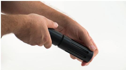
Unscrewing protective screen from the probe body.
